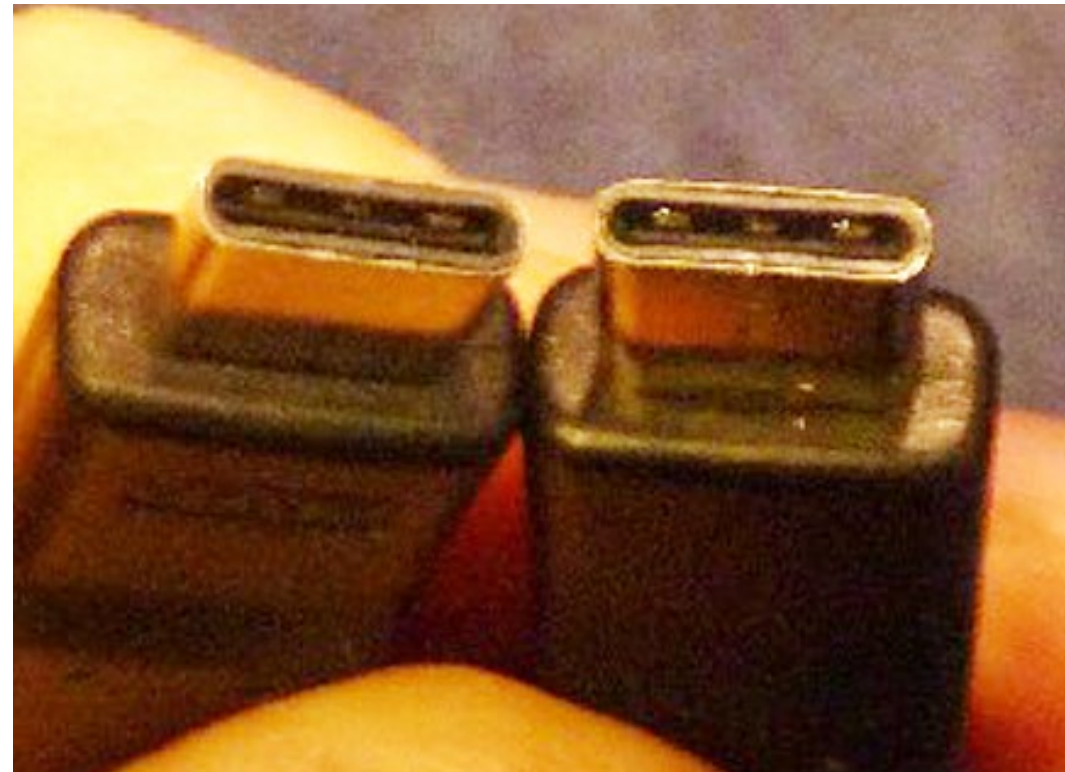
Figure 2. A USB Type-C cable can have Type-C connectors on both ends, making it easy to use.
