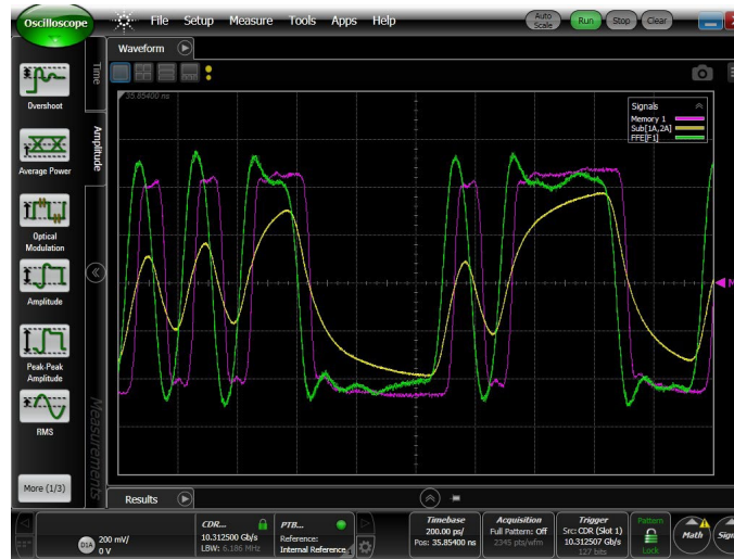
Figure 2. BertScope PRBS7 output (magenta); signal at PCB trace output (yellow); FIR filter output (green)
